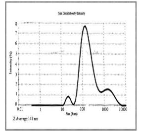
Figure 3. The size of silver nano particles obtained From leaves of *Portulaca oleracea.L*.
