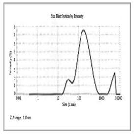
Figure 2. The size of silver nanoparticles obtained from stem of *Portulaca oleracea.L.*
