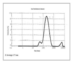
Figure 4. The size of silver nano particles obtained from root of *Portulaca oleracea.L.*
