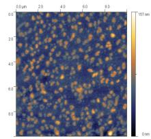
**Figure 6.** The AFM images of silver nanoparticles in root extract of *Portulaca oleracea.L.*
