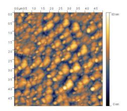
**Figure 7.** The AFM images of silver nanoparticles in stem extract of *Portulaca oleracea.L.*
