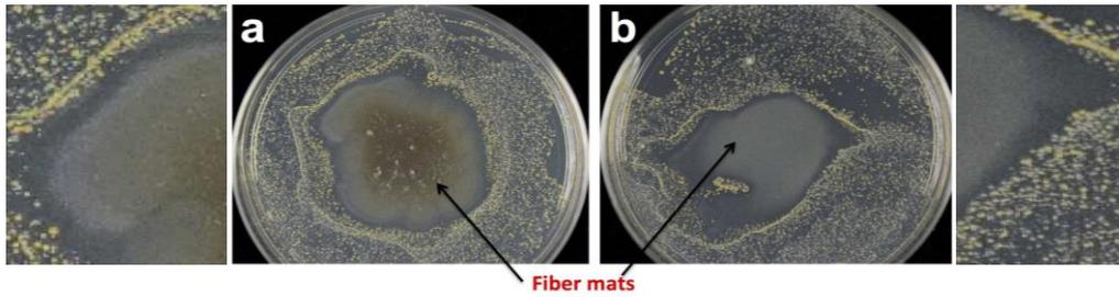
Fig 4. Antibacterial effect (a) Chitosan-0.2 wt %AgNPs with *Staphylococcus* bacteria and a (b) Chitosan-0.8 wt % CA sample with *Staphylococcus* bacteria. The whitish and yellowish colors surrounding the mats indicate the presence of the *Staphylococcus* bacteria. The images shown to the right and left of (a) and (b) show a magnified section of the inhibition zone. The bacteria does not penetrate the mats
