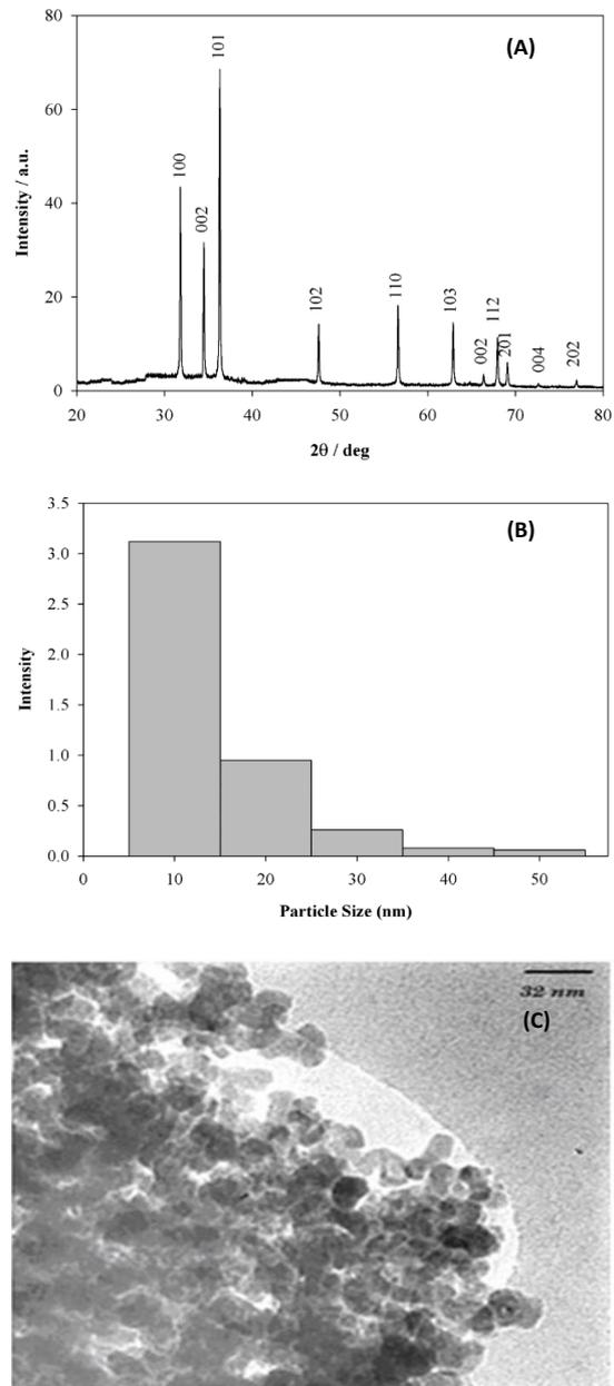
Fig 1. Characterizations of ZnO nanoparticles. X-ray diffraction patterns (A), Particle size distribution of ZnO nanoparticles (B), TEM image (C)
