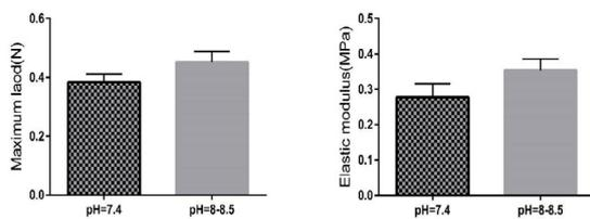
Fig 4. Mechanical properties of compressed hydrogels which were made in pH= 7.4 and pH=8.5. (left) Maximum load; (right) Elastic modulus. There were significant differences in maximum load and elastic modulus between hydrogels were made in pH=7.4 and 8.5 groups ( $p < 0.05$ ) ( $n=5$ )
