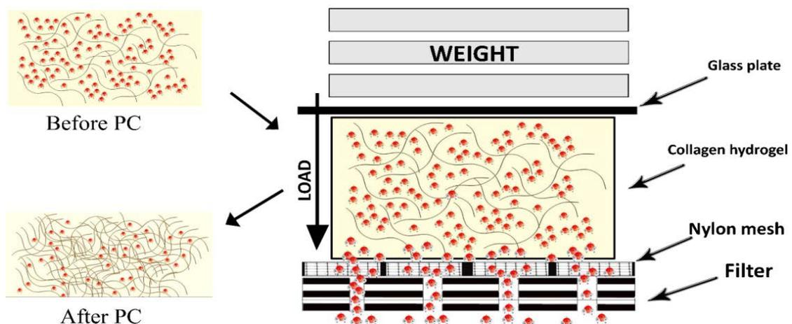
Fig 1. Plastic compression (PC) process. Schematic diagram showing plastic compression of collagen hydrogel including loading and blotting elements, and nylon meshes. Red bullets indicate water molecules
