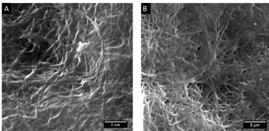
Fig 5. SEM images of collagen hydrogels. Overview of compressed collagen hydrogels made at pH=7.4 (A) and pH=8.5 (B)
