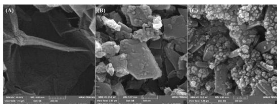
Fig 4. SEM images of GO (a),  $\beta$ -CD-GO (b)  $\beta$ -CD-GO-EDTA- $\text{Fe}_3\text{O}_4$ -SN38 (c)
