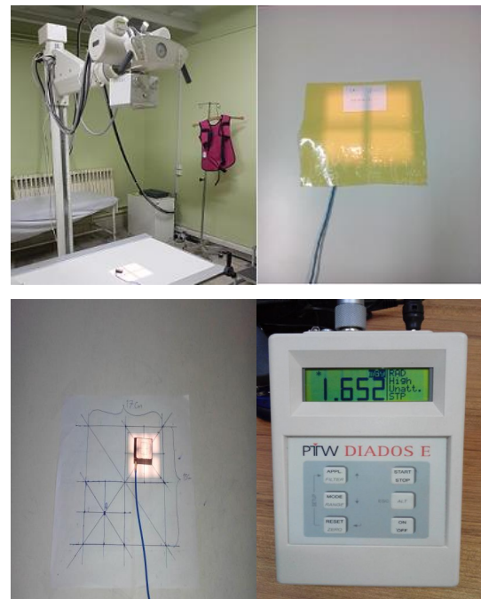
Fig 1. The photo of X-ray tube, setup of dosimeter and nano Bi 2 O 3 shield to measure dose reduction ability and uniformity.
