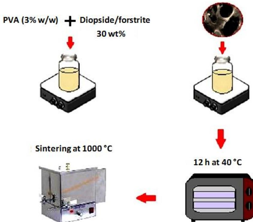
Fig 1. Fabrication procedure of the HA- nano- Diopside/Forstrite composite scaffold
