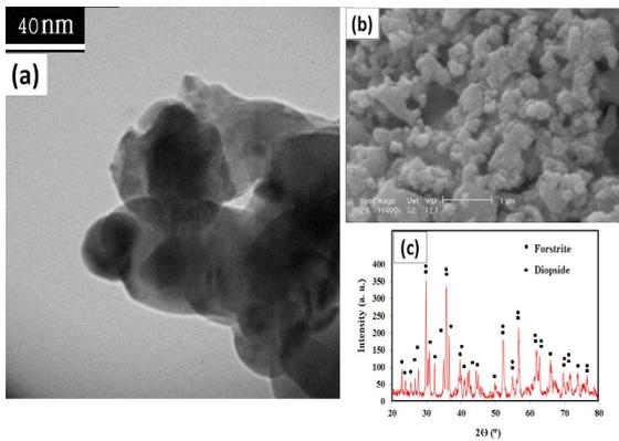
Fig 2. a (TEM micrograph, b) SEM micrograph and c) XRD pattern of nano-Diopside/Forstrite composite powder
