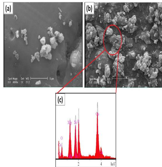
Fig 4. SEM micrograph of a( HA, b) HA- nano-Diopside/Forstrite composite scaffold and c) EDS spectrum of HA- nano-Diopside/Forstrite composite scaffold after 21 days soaking in SBF
