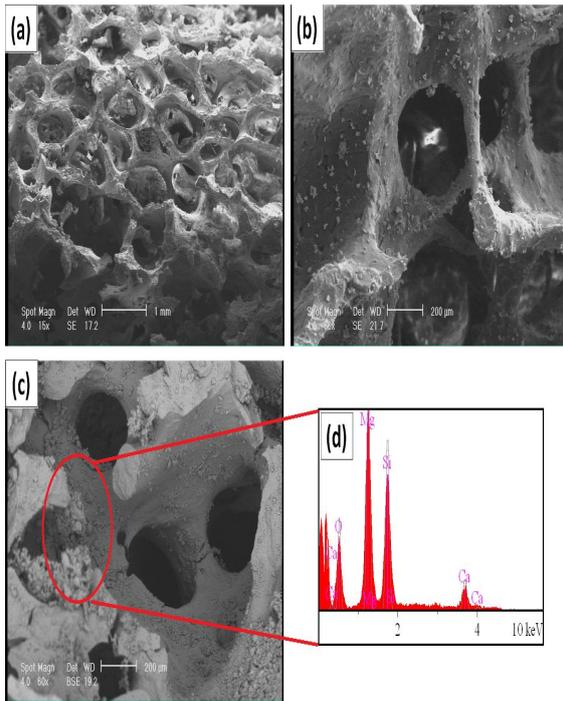
Fig 3. a-c( SEM micrograph and d) EDS spectrum of HA- nano-Diopside/Forstrite composite scaffold
