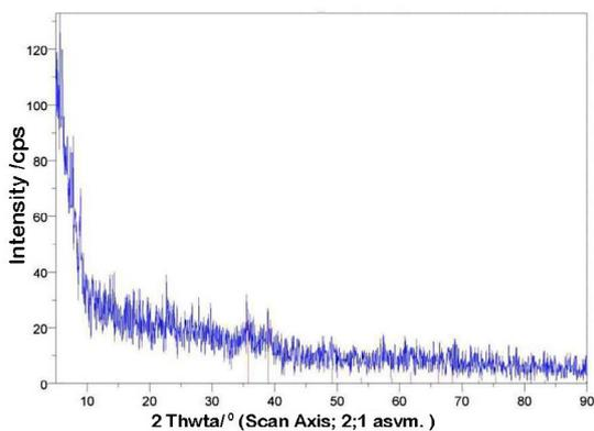
Fig 3. X-ray Diffraction Pattern of CuO/Epoxy Nanocomposite
