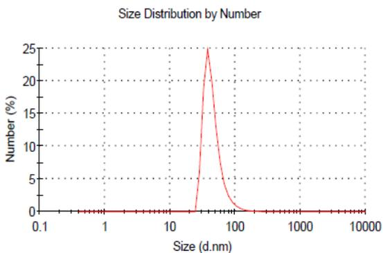
Fig 2. Size Distribution of CuO Nanoparticles Based on Number
