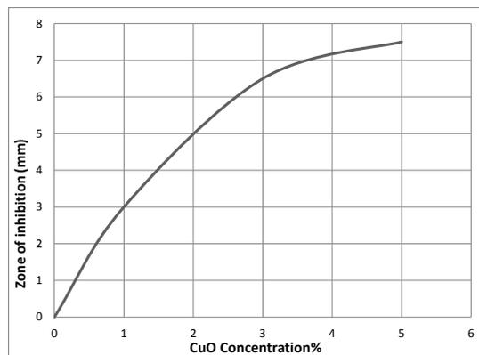
Fig 6. Curve of Inhibition Zone of CuO/Epoxy Nocomposite
