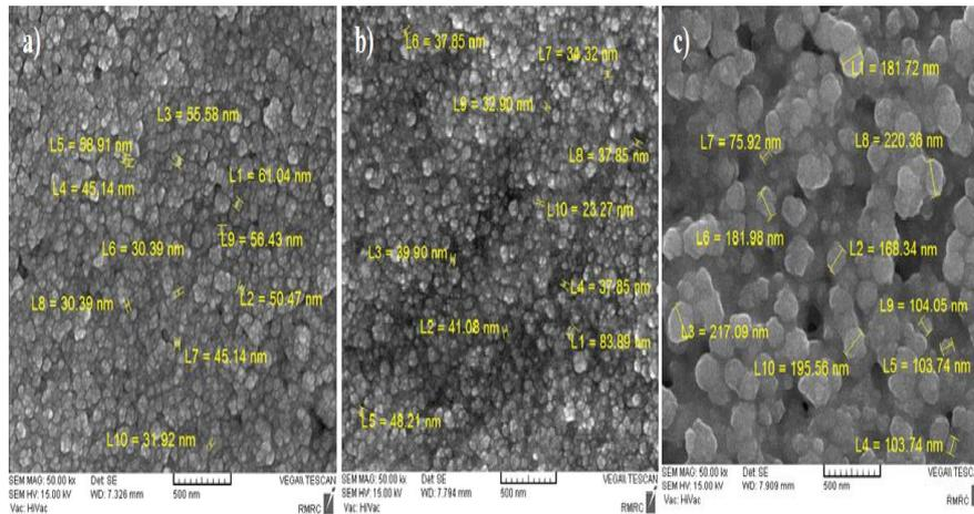
Fig 4. SEM Image of CuO/Epoxy Nanocomposite; a) 1% Concentration; b) 3% Concentration; c) 5% Concentration
