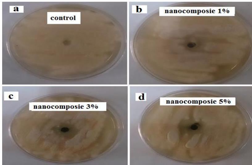
Fig 5. Inhibition Zone; a) Control Sample; b) 1% CuO/Epoxy Nanocomposite; c) 3% CuO/Epoxy Nanocomposite; d) 5% CuO/Epoxy Nanocomposite
