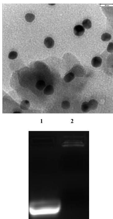
Fig 1 (a). TEM image of synthesized AuNPs. (b). Assessment of OTC aptamer attachment on the surface of AuNPs. Lane 1: OTC aptamer, lane 2: OTC aptamer-modified AuNPs
