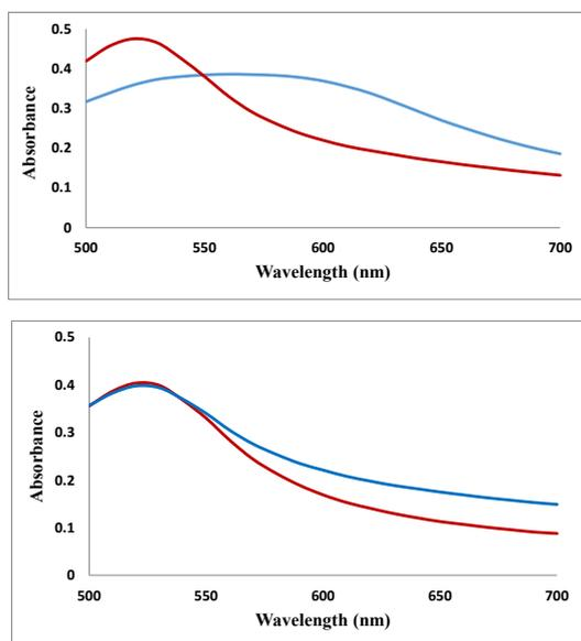
Fig 2. (a). Absorbance spectra of aptasensor in the presence (blue curve) and absence of OTC (red curve) in water sample. (b). Absorbance spectra of aptasensor in the presence (blue curve) and absence of OTC (red curve) in milk sample
