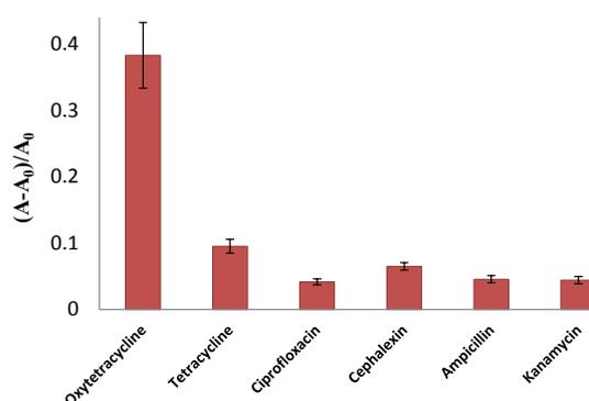
Fig 4. The response of designed aptasensor to OTC and other antibiotics in milk
