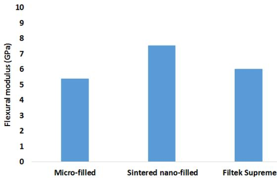
Fig 4. Mean flexural modulus of materials [28]
