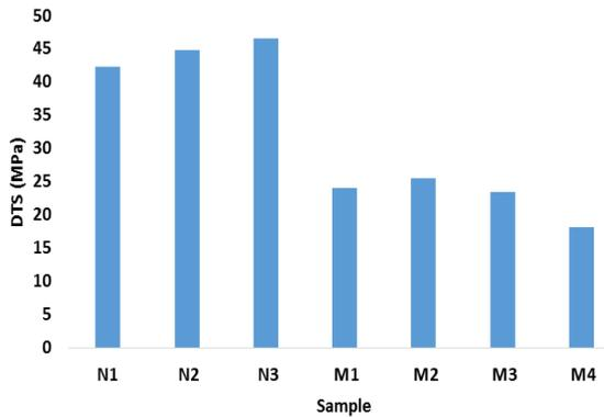
Fig 7. Mean diametral tensile strength of samples containing micro- and nano-sized materials [32]
