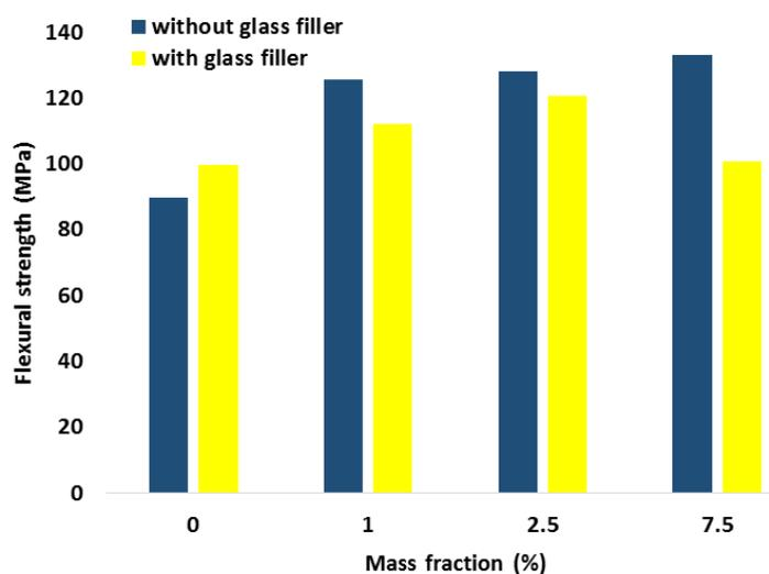
Fig 8. Flexural Strength and Mass Fraction of Nano-materials [35]
