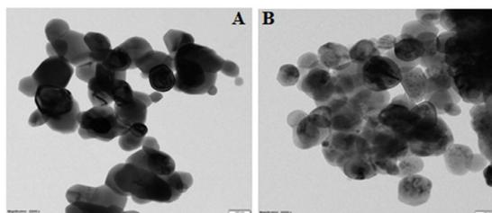
Fig 4. (A) TEM images of chemically synthesized ZnO nanoparticles, (B) TEM images of green synthesized ZnO nanoparticles
