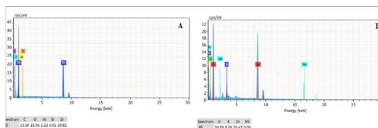
Fig 3. EDAX spectrum of (A) chemically synthesized ZnO nanoparticles, (B) green synthesized ZnO nanoparticles
