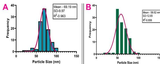
Fig 5. Particle size distribution graph of (A) chemically synthesized ZnO nanoparticles, (B) green synthesized ZnO nanoparticles
