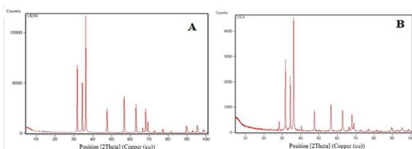
Fig 6. (A) XRD images of (A) chemically synthesized ZnO nanoparticles, (B) green synthesized ZnO nanoparticles
