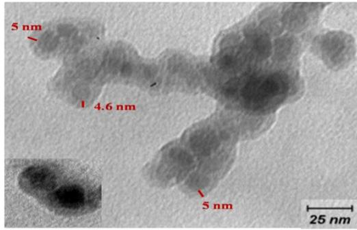
**Figure 4.** TEM image of the magnetite-silica core/shell nanocomposite.
