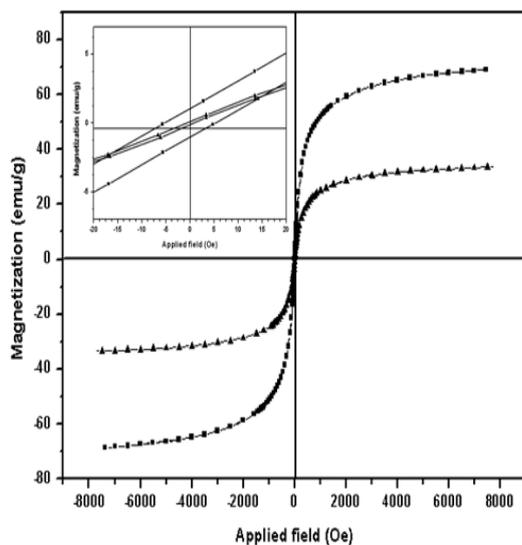
**Figure 6.** Magnetization curves of  $\text{Fe}_3\text{O}_4$  NPs (■) and  $\text{Fe}_3\text{O}_4@\text{SiO}_2$  nanocomposite (▲) at 300K. Inset: the enlarged curves from -20 to 20 Oe.
