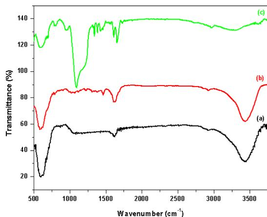
**Figure 5.** FT-IR spectra of: (a) pristine MNPs, (b) citrate-modified MNPs and (c) Fe<sub>3</sub>O<sub>4</sub>@SiO<sub>2</sub> nanocomposite.
