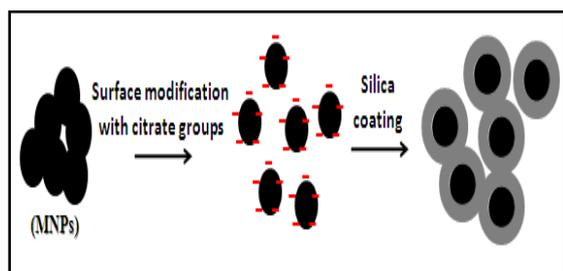
**Figure 1.** Schematic presentation of the synthesis process of magnetite-silica nanocomposite.
