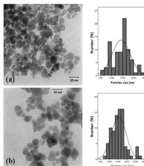
**Figure 3.** TEM images of MNPs (a) before and (b) after surface modification with 0.5M trisodium citrate solution.
