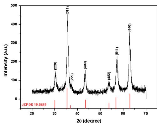
**Figure 2.** X-ray diffraction pattern of  $\text{Fe}_3\text{O}_4$  nanoparticles.
