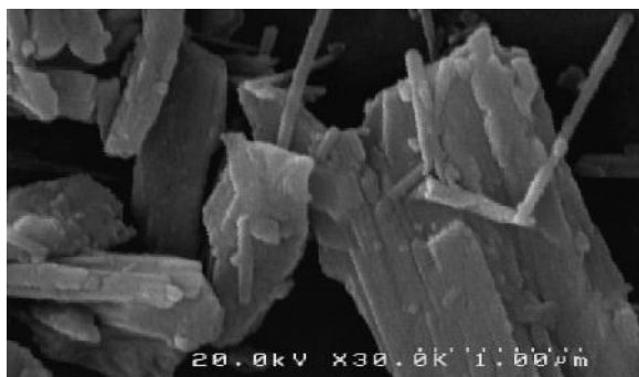
Figure 1. A scanning electron micrograph of MnO 2 microparticles.
