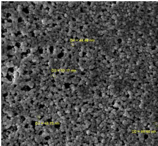
Fig.1. SEM image of chitosan nanoparticles
