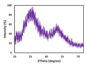
Fig. 2. The XRD pattern of Se-NPs
