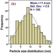
Fig. 5. TEM (a) and Particle size distribution curve according to TEM image (b)
