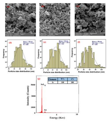
Fig. 6. FESEM images (a-c), Particle size distribution curve according to FESEM images (d-f), and EDX analysis of Se-NPs (g)
