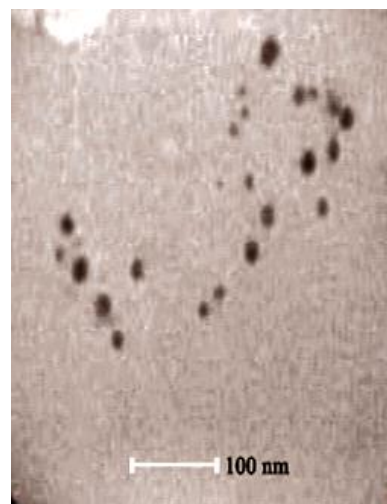
Figure 3. TEM micrograph of silver particles synthesized by A. parasiticus (scale bar: 100 nm).
