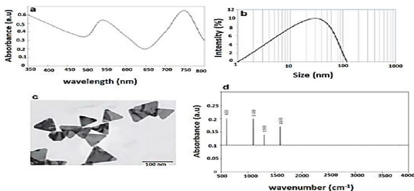
**Figure 1.** Characterization of triangular gold nanoparticles. UV-VIS spectrum (a), DLS graph (b), TEM image of triangular gold nanoparticles (c), FTIR peaks (d) of triangular gold nanoparticles at concentration of 32  $\mu\text{g/mL}$ . For better interpretation, we omitted the noise signals, and only main peaks were shown.
