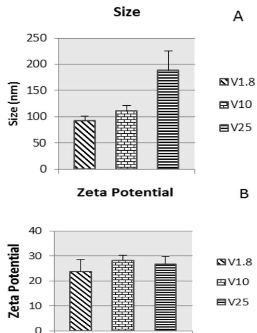
Figure7. A) Size B) Zeta potential of polyplexes at C/P=2.
