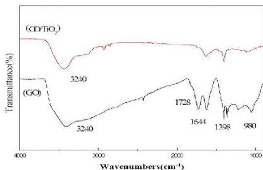
Fig. 2. FT-IR spectra of GO and GO/TiO<sub>2</sub>
