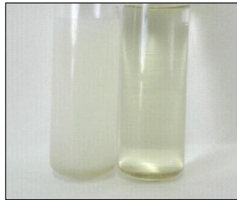
Fig. 2. The prepared nanoemulsions (right : nanoemulsions with NaCl 0.1) M and left: nanoemulsions with NaCl 0.5 M
