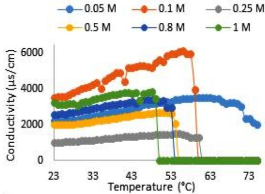
Fig. 1. The conduction chart by temperature related to nanoemulsions having various concentrations of NaCl
