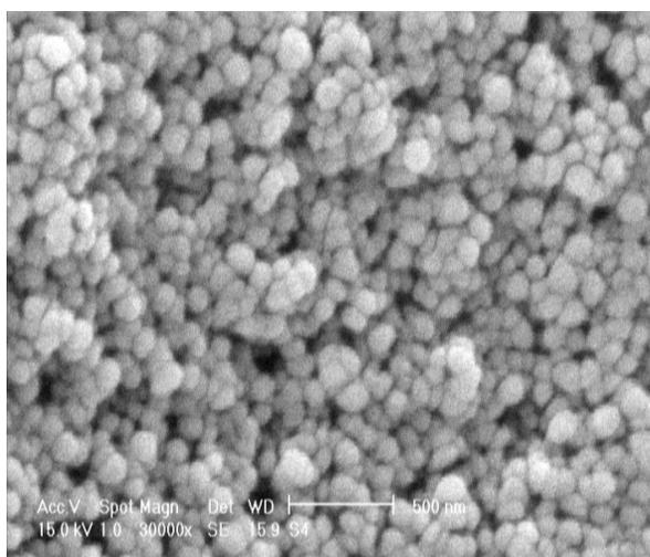
Fig. 3. SEM micrograph of irinotecan loaded PLGA nanoparticles (S9)
