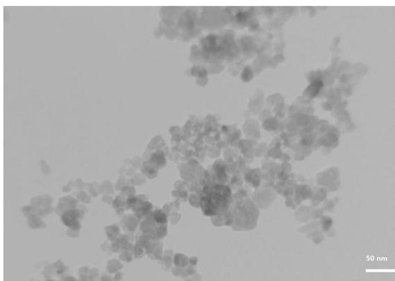
Fig. 2. Transmission Electron Microscope of ZnS:Ag QDs
