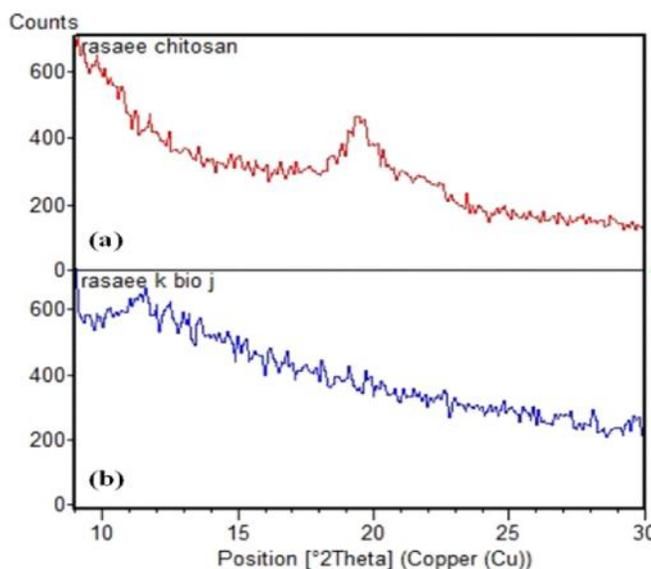
Fig. 3. XRD patterns: (a) Chitosan and (b) Biosynthesized CNPs
