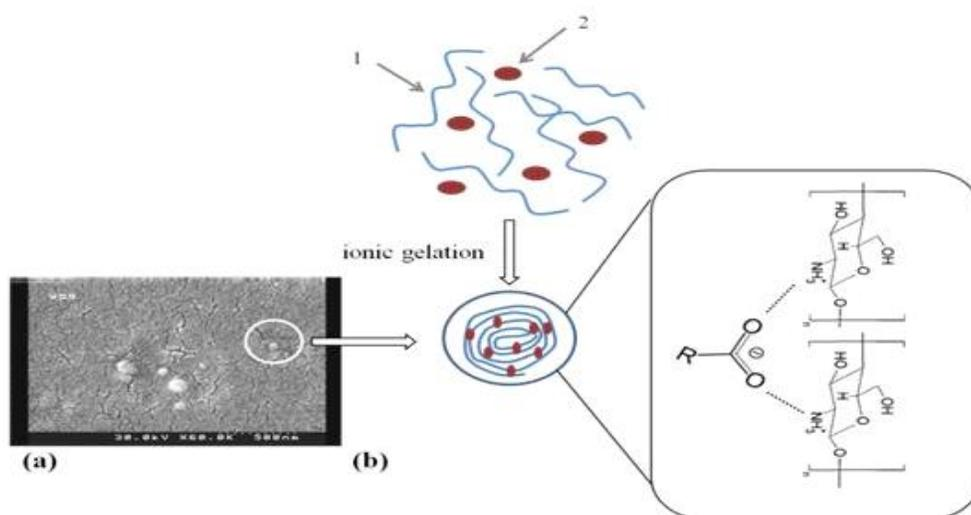
Scheme. 1. Proposed mechanism to form of chitosan nanoparticles by ionotropic gelation: (a) SEM image of the biosynthesized nanoparticle, (b) schematic illustration of the chitosan-anion complex. 1 chitosan and 2 negatively charged functional groups of *O. basilicum* leaf extract such as  $\text{COO}^-$
