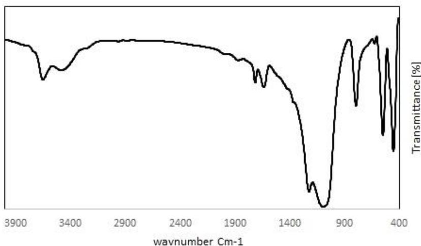
Fig. 3. The FT-IR transmission spectra for ZSM-5 zeolite without organic template
