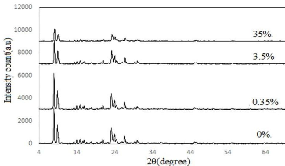
Fig. 2. XRD pattern of binary hybrid composites of nano chitosan/ ZSM-5 with chitosan content of 35%, 3.5%, 0.35%, 0%
