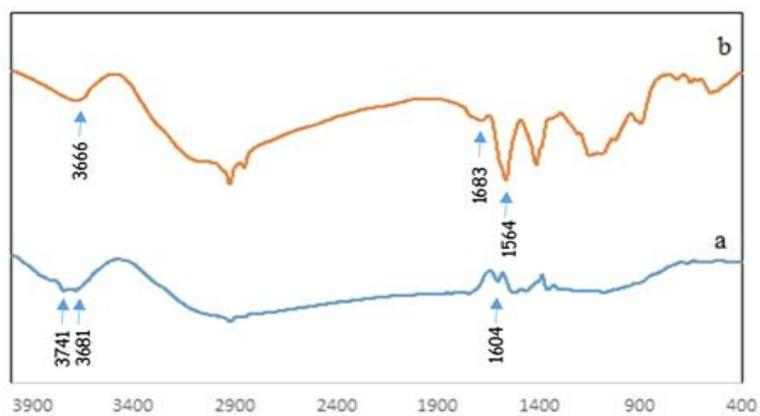
Fig. 5. FT-IR spectra of (a) chitosan and (b) chitosan nano particles
