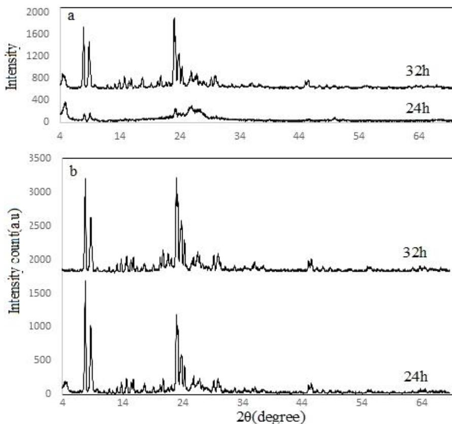
Fig. 1. Effect of crystallization without seed (a), with seed (b) on crystallinity of as-synthesized ZSM-5
