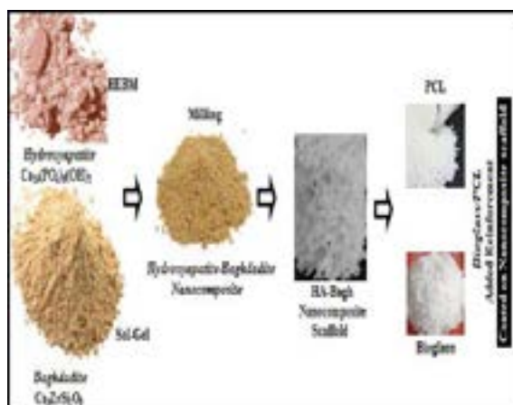
Fig. 1. Schematic of HA-Bagh nanocomposite coated with BG/PCL reinforcement preparation
