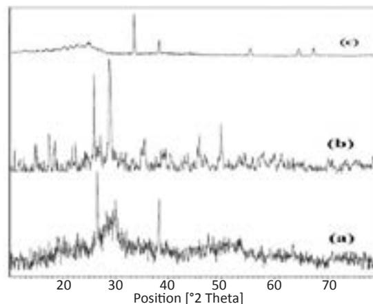
Fig. 1. XRD pattern of a) Cd(OAc)<sub>2</sub> nanostructure and b) CdO/GrO nanolayer sublimated at 330 °C for 120 min and c) XRD pattern of graphene
