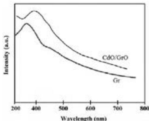
Fig. 7. UV-Vis spectra of Graphene and CdO/GrO nanolayers
