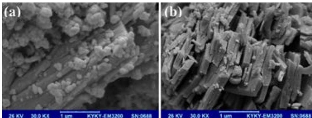
Fig. 2. SEM images of the Cd(OAc)<sub>2</sub> sublimated at 130 °C (a) and CdO/GrO nanolayers sublimated at 330 °C
