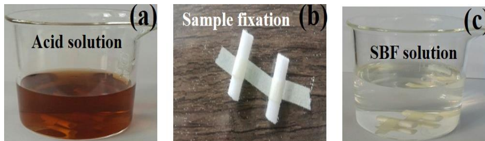
Fig 7. Results of biological testing of artificial bio-nanocomposite made by 3D printing soaked in a) Acid solution, b) Sample fixation in saline solution, and c) SBF solution for 21 days
