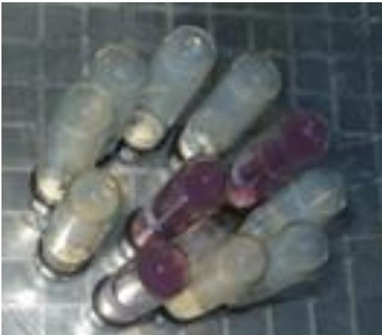
Fig 3. The arrangement of the MAGIC-f gel tubes prepared to be irradiated by a linac 18 MV beam
