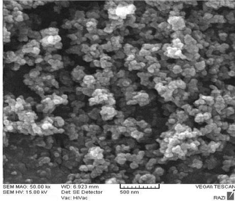
Fig 1. Scanning Electron Microscopy Image of nFe2O3 Dry Powder
