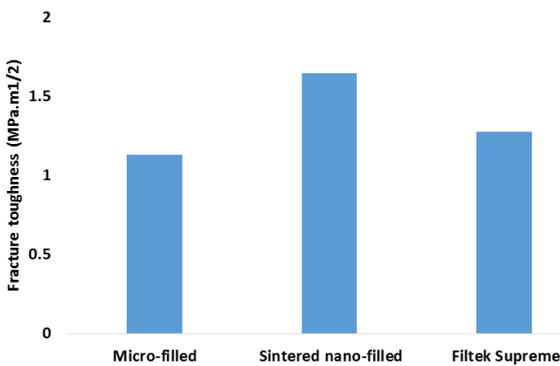
Fig 5. Mean fracture toughness of materials [28]
