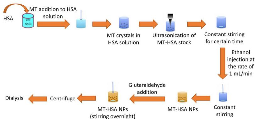
Fig 1. Preparation of MT-HSA NPs using ultrasonication and desolvation methods
