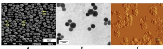
Fig 3. (a) SEM, (b) TEM and (c) AFM images of MT-HSA NPs
