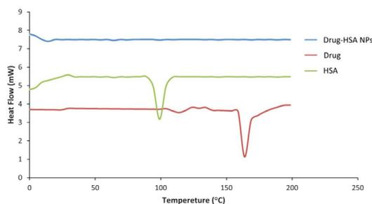
Fig 4. DSC of pure MT, HSA and MT- HSA NPs
