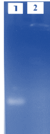
Fig 4. Gel electrophoresis assay analysis of aptamer conjugated to AuNPs. Lane1: aptamer, lane2: aptamer conjugated to AuNPs
