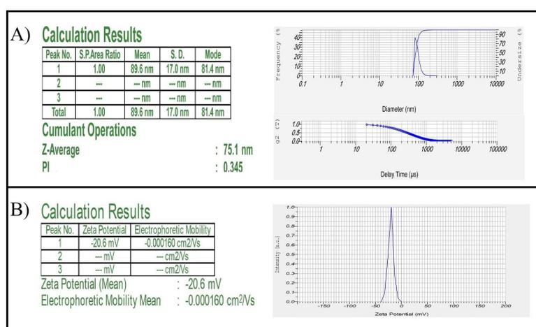
Fig 2. A, the average size of nanoparticles after loading of HH extract and adding DSPE-PEG obtained from DLS. B, the average zeta potential (mV) of Nio-HHE after adding DSPE-PEG obtained from DLS
