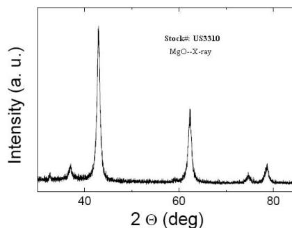
Fig. 2. X-ray pattern of MgO NP. Diffraction angle is between 35° and 85°
