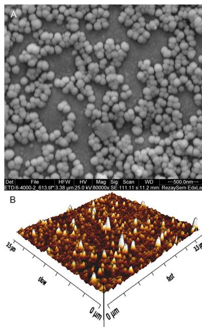
Fig. 4. A) Scanning electron microscopy (SEM) photograph of niosome containing curcumin. B) Atomic force microscopy (AFM) photograph of niosome containing curcumin
