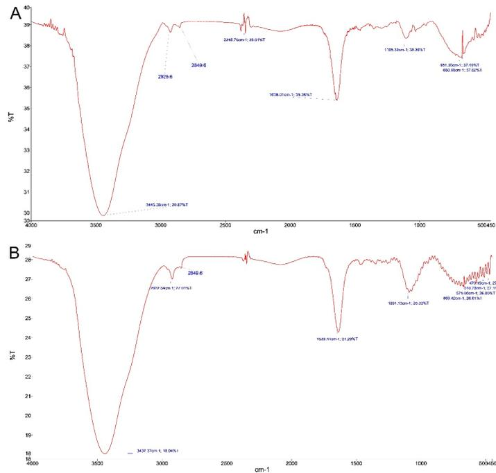
Fig. 5. FTIR spectra of optimum formula (F1) in before (A) and after curcumin loading (B)
