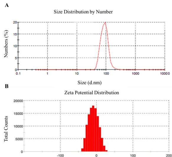
Fig. 2. A) Data obtained from the analysis of a niosomes by a zeta-sizer. According to these data, the average size of nanoparticles is 90.08 nm and their dispersion index is 0.236. B) Average of zeta potential of niosomes. The data show that the zeta potential of nanoparticles is  $-8.21 \pm 3.46$  mV
