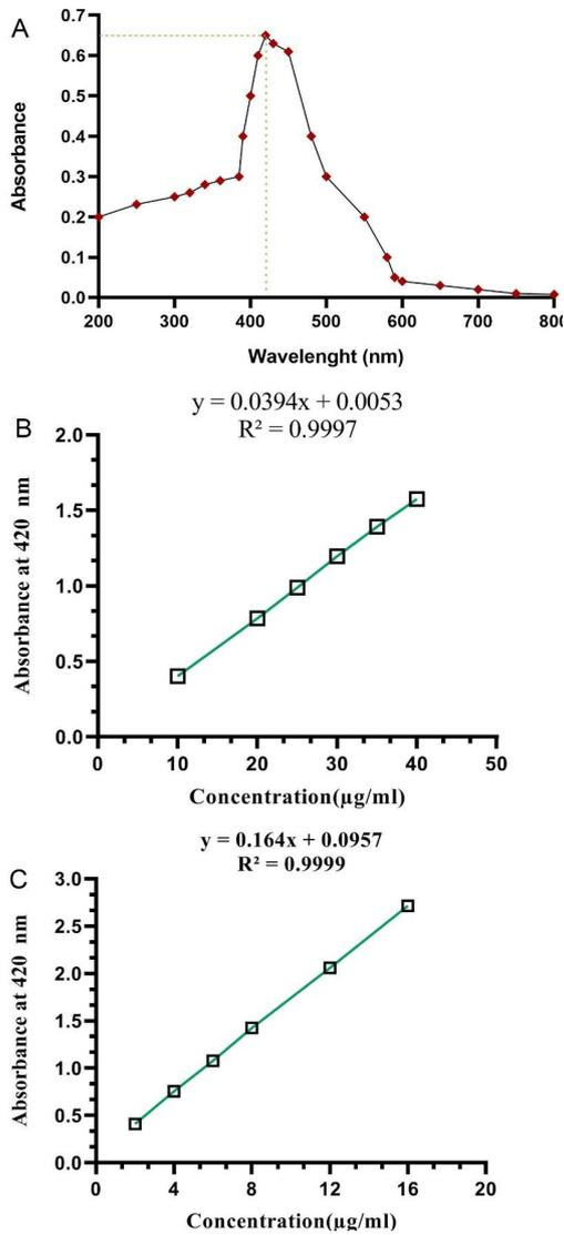
Fig. 1. A) Absorption spectrum of curcumin at wavelengths of 200 to 800 nm. The maximum absorption value is at 420 nm. B) The standard curve of curcumin in PBS buffer is derived from the evaluation of the absorption spectra in different concentrations of curcumin at its maximal absorption wavelength. C) The standard curve of curcumin in isopropyl buffer is derived from the evaluation of the absorption spectra in different concentrations of curcumin at its maximal absorption wavelength
