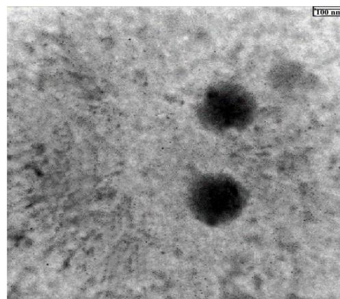
Fig. 2. Transmission electron microscopy image of luteolin nanoemulsion (scale: 100 nm)
