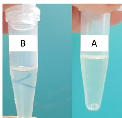
Fig. 5. Phase separation in luteolin-loaded nanoemulsion. A) before centrifugation and B) after centrifugation
