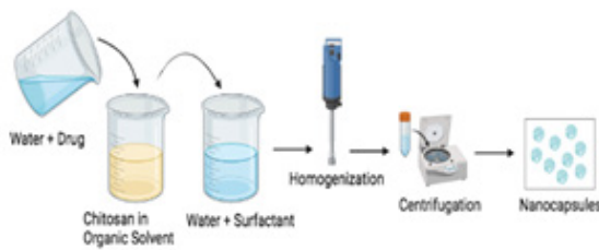
Fig. 6. Schematic illustration of polymeric nanocapsule synthesis using the double emulsion method (Created in Biorender.com)
