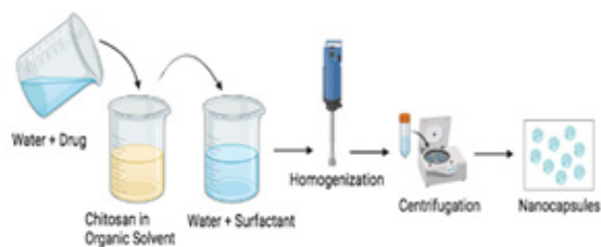
Fig. 6. Schematic illustration of polymeric nanocapsule synthesis using the double emulsion method (Created in Biorender.com)
