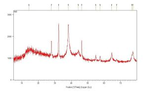
Fig. 4. XRD pattern of the synthesizes AgNPs in green synthesis
