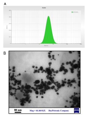
Fig. 3 A: Particle size distribution of synthesized AgNPs using aqueous extract of Pistacia vera, B: The morphology of AgNPs was imaged by transmission electron microscope (TEM)
