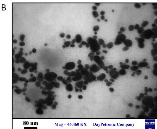
Fig. 3 A: Particle size distribution of synthesized AgNPs using aqueous extract of Pistacia vera, B: The morphology of AgNPs was imaged by transmission electron microscope (TEM)
