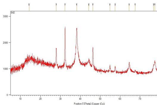
Fig. 4. XRD pattern of the synthesized AgNPs in green synthesis
