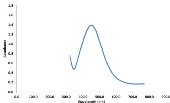
Fig. 2. UV- visible spectroscopy of green synthesized silver nanoparticles
