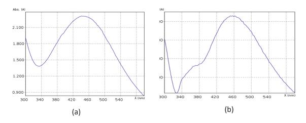
Fig 1. UV-visible absorption spectra of (a) AgNPs, and (b) Li-AgNPs.
