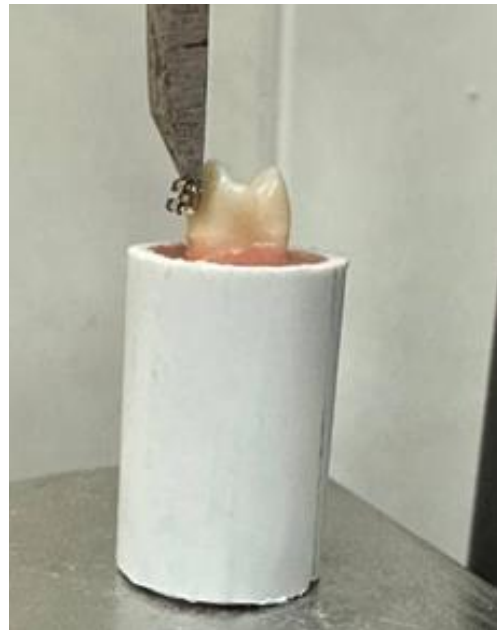
Fig. 2. Loading of the bracket under shear force in SBS testing setup
