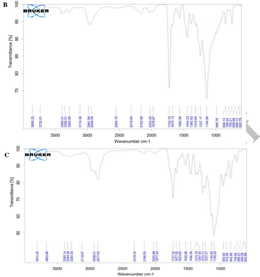
Fig. 1. FTIR spectrum graphs for (A) CP, (B) ERS100, and (C) a mixture of CP and ERS100 at ratio 1:1.
