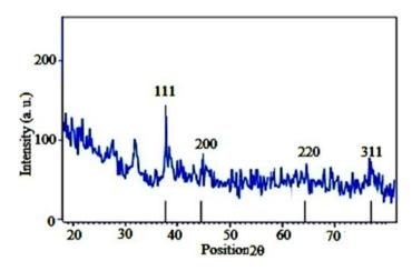
Fig. 4. X-ray diffraction pattern of silver nanoparticles synthesized by Streptomyces somaliensis isolate G
