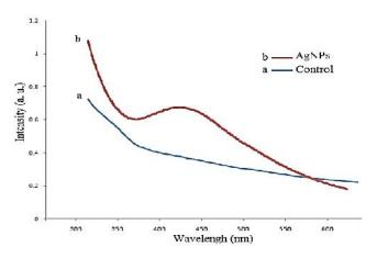
Fig. 2. The UV-Vis spectrometer of silver nanoparticles synthesized by *S. somaliensis* isolate G After reactions with the *S. somaliensis* isolate G for 24 h. Presence of a strong peak with maximum absorbance at 450 nm is prominent
