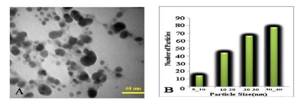
Fig. 3. (A) TEM micrograph recorded of an aqueous solution incubated with *Streptomyces somaliensis* isolate G with Ag<sup>+</sup> ions for 24 h. (B) Histogram of size distribution of the silver nanoparticles from TEM analysis
