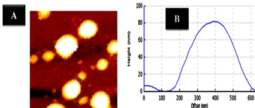
Fig. 1. AFM image of PLGA-DOX-Cro NPs (F8) obtained in the tapping mode (A). Height profile of PLGA-DOX-Cro NPs (B)
