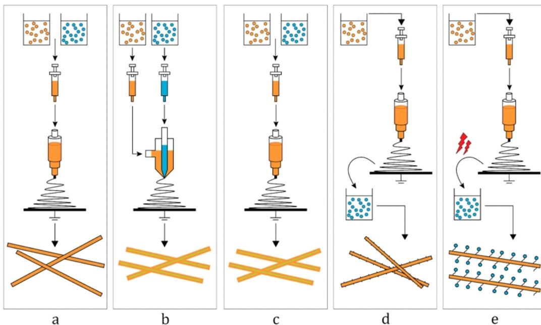
Fig. 2. Schematic picture of different methods of drug incorporation into nanofibers
