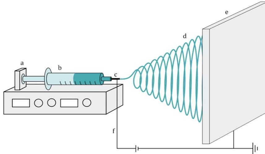
Fig. 1. Schematic picture of a typical electrospinning setup
