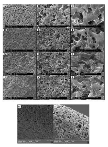
Fig 3. Scanning electron micrographs of pure PCL (A-C), and PCL nanofibrilliated chitosan nanocomposits, NC2.5 (D-F), NC5 (G-I), NC10 (J-L), in different magnifications. M and N are representative for cross-sectional micrographs of NC5 sample
