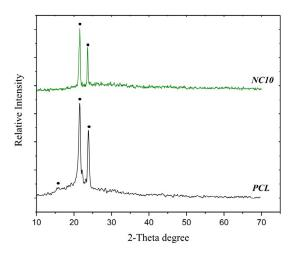
Fig 6. XRD patterns of PCL and NC10 samples. The signs show the characteristic peaks concerning each sample
