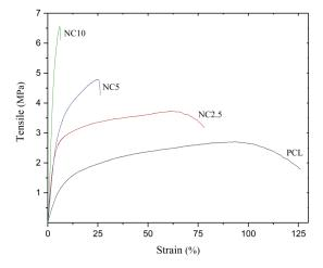
Fig 5. Stress-strain curves of PCL and NC composite samples
