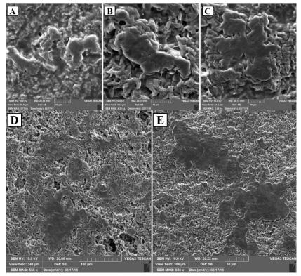
Fig 10. SEM projections of adhered cells on the scaffolds: (A) PCL, (B) NC5, (C) NC10 after 12h of incubation. D and E respectively show NC5 and NC10 cell-containing scaffolds in lower magnifications which Cell-mass regions are clearly distinguishable
