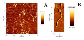
Fig 1. AFM image of (a) chitosan nanofibrils (b) an individual chitosan nanofibril
