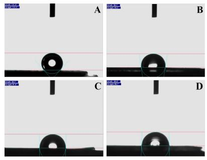
Fig 7. Contact angle measurement for PCL (A), NC2.5 (B), NC5 (C), and NC10 (D) samples
