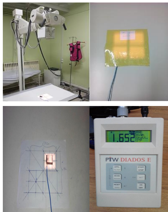
Fig 1. The photo of X-ray tube, setup of dosimeter and nano Bi 2 O 3 shield to measure dose reduction ability and uniformity. A: Radiography device with probe of dosimeter, B: Physical dosimetric map for 5 recording placements of dose in air, C: Similar physical dosimetric map for 5 recording placements with shield, D: Dosimetric device called DIADOS E (PTW) that measure the dose (μGy) for showing dose reduction uniformity
