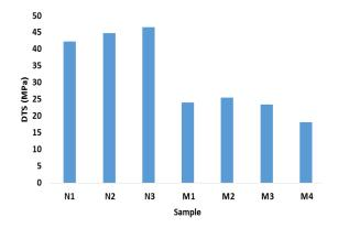
Fig 7. Mean diametral tensile strength of samples containing micro- and nano-sized materials [32]
