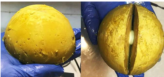
Fig 5. Oil-gelatin phantom of breast with fat, glandular, and tumor tissues
