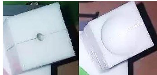
Fig 2. Cube used for fabrication of tumor tissues (hole was used for mixture injection)
